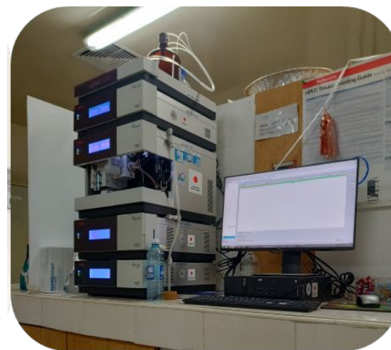
Ultimate 3000 Dionex (Thermo Scientific) with PDA detector
